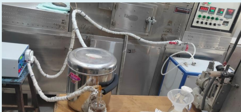
Figure 3: Customized &continuous microwave processing
